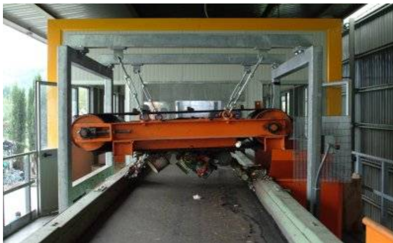
Figura 5.2.2.3-7: Separator magnetic automat feroase
